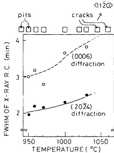
FIG. 4. Variation of FWHM of XRC (average of two different positions in the same film) and the appearance of the GaN film with the growth temperature.  $\langle 11\bar{2}0 \rangle$  cracks are seen at higher temperatures and pits at lower temperatures.
