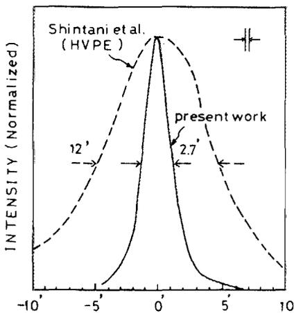
FIG. 3. X-ray rocking curve for (0006) diffraction from GaN grown at 970  $^{\circ}\text{C}$  with the AlN buffer layer. Dotted line shows data obtained by HVPE.<sup>11</sup>
