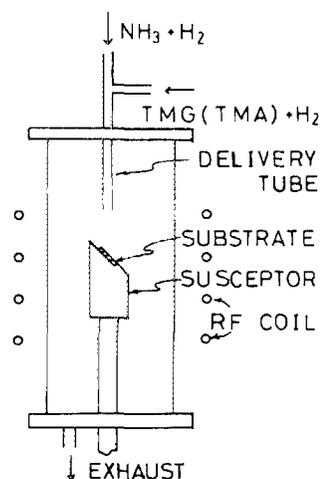
FIG. 1. Schematic drawing of the reactor part of the MOVPE system.
