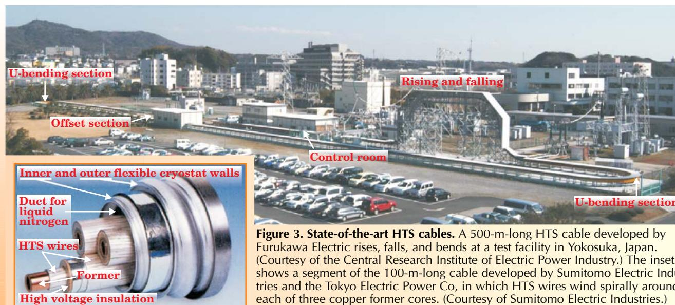
**Figure 3. State-of-the-art HTS cables.** A 500-m-long HTS cable developed by Furukawa Electric rises, falls, and bends at a test facility in Yokosuka, Japan. (Courtesy of the Central Research Institute of Electric Power Industry.) The inset shows a segment of the 100-m-long cable developed by Sumitomo Electric Industries and the Tokyo Electric Power Co, in which HTS wires wind spirally around each of three copper former cores. (Courtesy of Sumitomo Electric Industries.)
