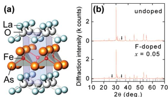
**Figure 1.** (a) Crystal structure of LaOFeAs. (b) Powder XRD patterns of undoped LaOFeAs and La[O<sub>1-x</sub>F<sub>x</sub>]FeAs:  $x = 0.05$ . Black bars at bottom show calculated Bragg diffraction positions of LaOFeAs. Arrows denote peaks due to impurity phases, FeAs (helimagnetic),<sup>13</sup> and LaOF.
